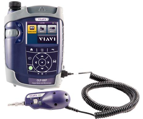
SmartClass Fiber tester with P5000i and patch-cord microscopes
