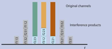
This interference phenomenon produces unwanted signals from three frequencies ( $f_{xyz} = f_x + f_y - f_z$ ) known as ghost channels. As three channels automatically induce a fourth, the term four wave mixing is used. FWM is problematic in systems using dispersion-shifted fibers (DSF). Wavelengths traveling at the same speed at a constant phase over long periods increase the effect of FWM.
