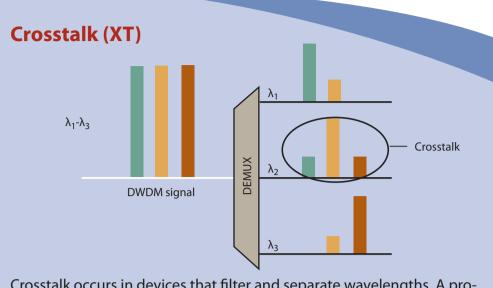
Crosstalk occurs in devices that filter and separate wavelengths. A proportion of optical power intended for a specific channel is found in an adjacent or different channel.
