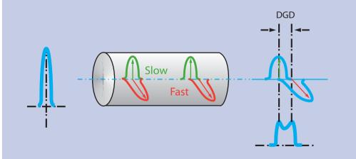
PMD refers to the effect when different polarization modes (fast axis and slow axis) of a signal statistically travel at different velocities due to fiber imperfections. The time difference is called Differential Group Delay (DGD).
