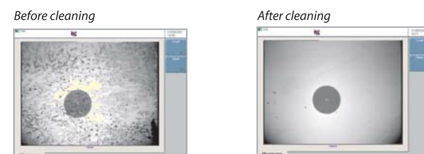
Fiber connectors should always be visually inspected before mating!
