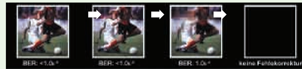
Digital video channels stay clear until FEC can no longer compensate for signal impairments
