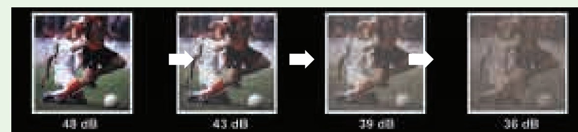
Analog signals degrade linearly with signal impairments
